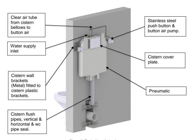
Figure 7: Typical installation layout
