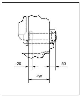
Figure 2:Horizontal flush pipe cutting instructions
